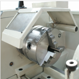
Chuck Guard With Safety Micro Switch
