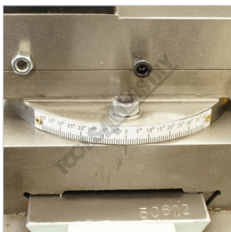
Compound Slide Angle Scale
