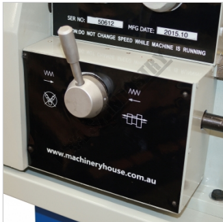
Directional Feed Control Lever
