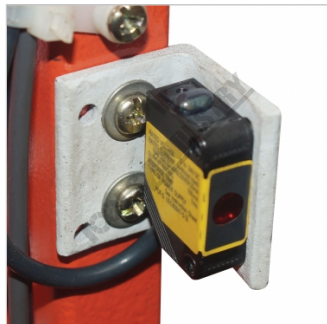
Safety Omron E3ZS Rear Light Sensor Guarding
