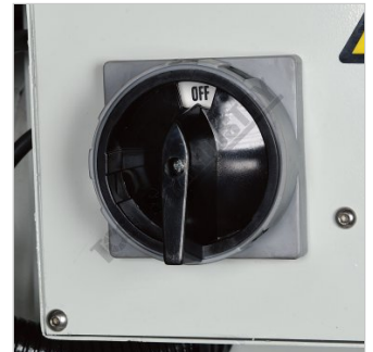
Main Isolation Switch
