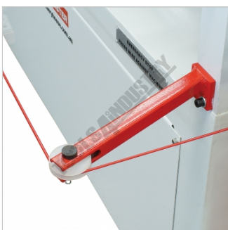
Safety Wire Interlock System
