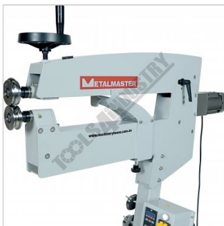
Adjustable Material Gauge at Full Depth
