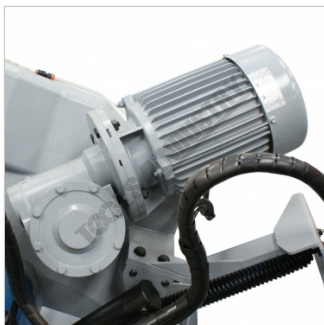
Motor and Gearbox Drive
