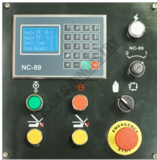
NC 89 Control Panel
