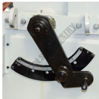
Rapid Blade Adjustment for Material Thickness
