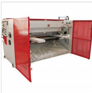
Rear guarding with safety sensors
