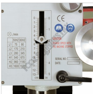
Quill Depth Stop Scale & Spindle Lock
