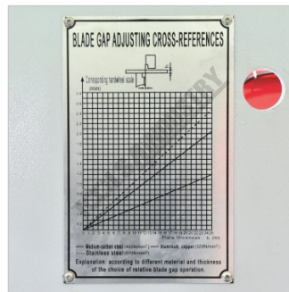
Blade Gap Adjustment Diagram
